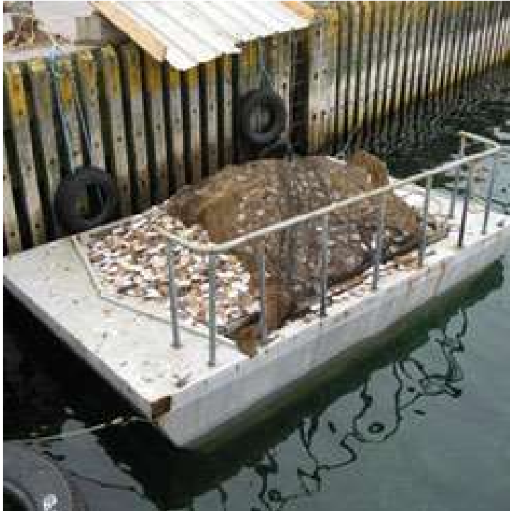
Figure 2 – Fish wastes on a barge. Note that spillage is possible so weather and wave conditions should be acceptable on the way to the dump-site to prevent loss of materials
